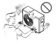
If strange sounds, or small or smoke comes from product. Turn the breaker off or disconnect the power supply cable.
